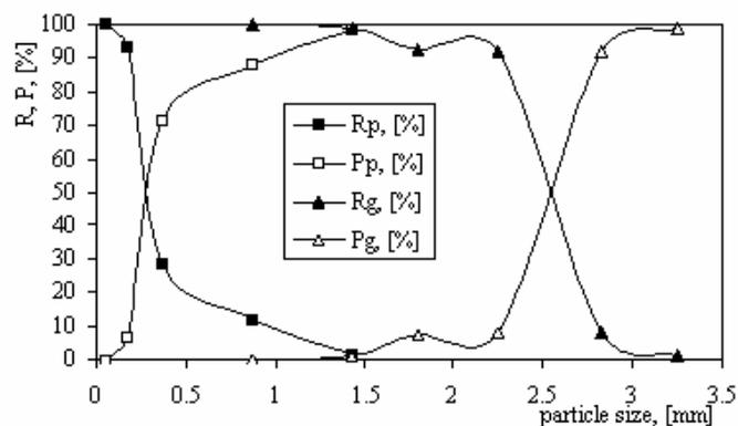
Fig. 4 – Particle size presentations in normal distributions for granular (g) and powdered (p) urea: the cumulative distributions (R – oversize, P – undersize).
