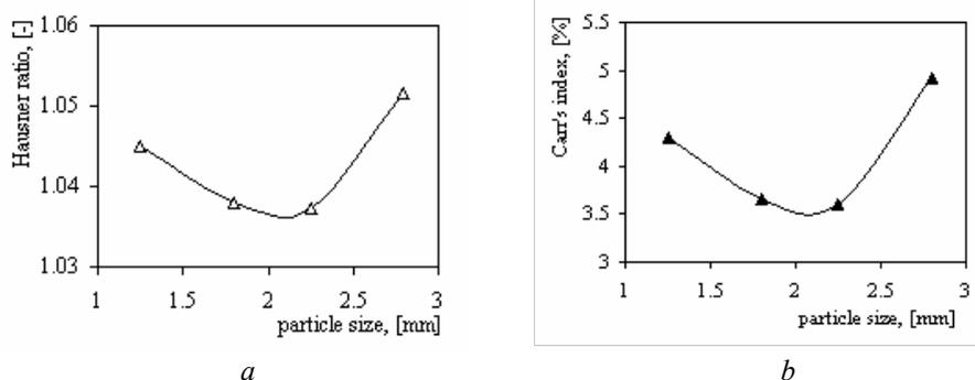
Fig. 7 – Effect of urea particle size on Hausner ratio (a) and Carr's index (b).
