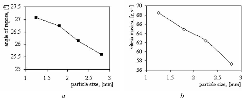
Fig. 8 – Effect of urea particle size on angle of repose (a) and flow rate (b).
