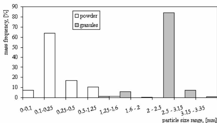
Fig. 3 – Particle size presentations in normal distributions for granular and powdered urea: histograms of frequency *versus* range size.
