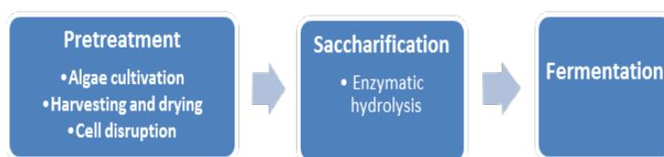
Fig. 3 – Main steps in the production of bioethanol from algal biomass.
