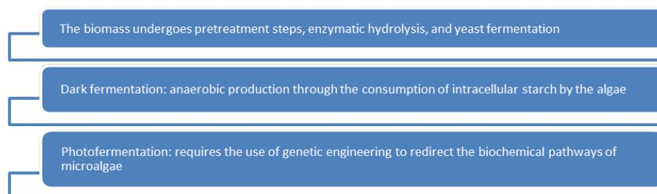
Fig. 2 – Schematic routes for bioethanol production from algae.
