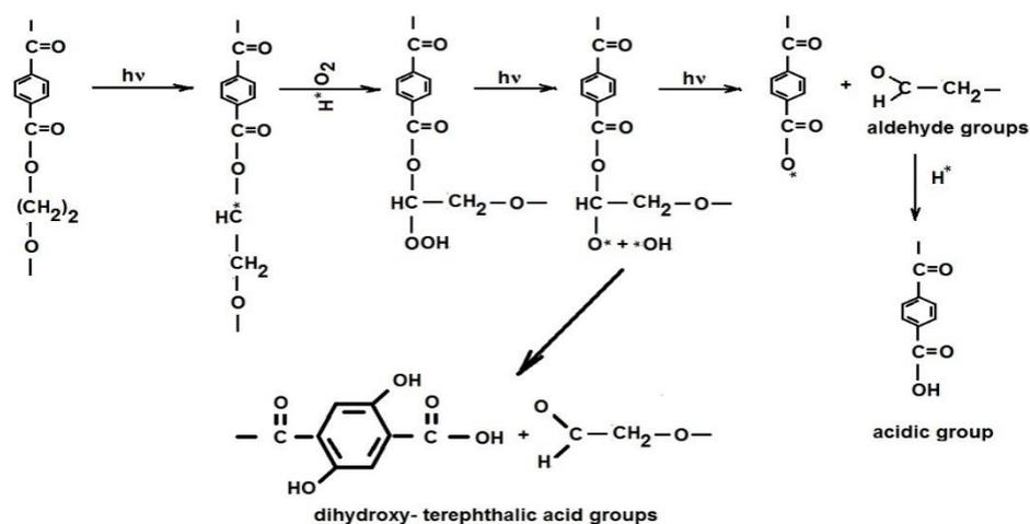
Fig. 1 – Surface functionalization PET mechanism with UV radiation action at  $\lambda = 254 \text{ nm}$ .
