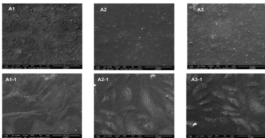
Fig. 5 – (SEM) images of immobilized modified PET films- for (2, 4, 6) gelatine A<sub>1</sub>, A<sub>2</sub>, A<sub>3</sub> followed by cell growth (A<sub>1-1</sub>, A<sub>2-1</sub>, A<sub>3-1</sub>)
