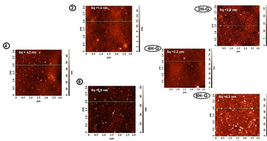
Fig. 2 – AFM 2D images (topography) obtained for UV functionalized polyethylene terephthalate films at various times and immobile with biomolecules.
