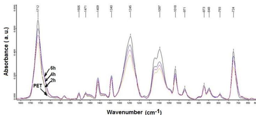
Fig. 3 – The FTIR-ATR spectra in the range of 1800-600  $\text{cm}^{-1}$  for UV-functionalized PET film at different irradiation times (2, 4, 6h).
