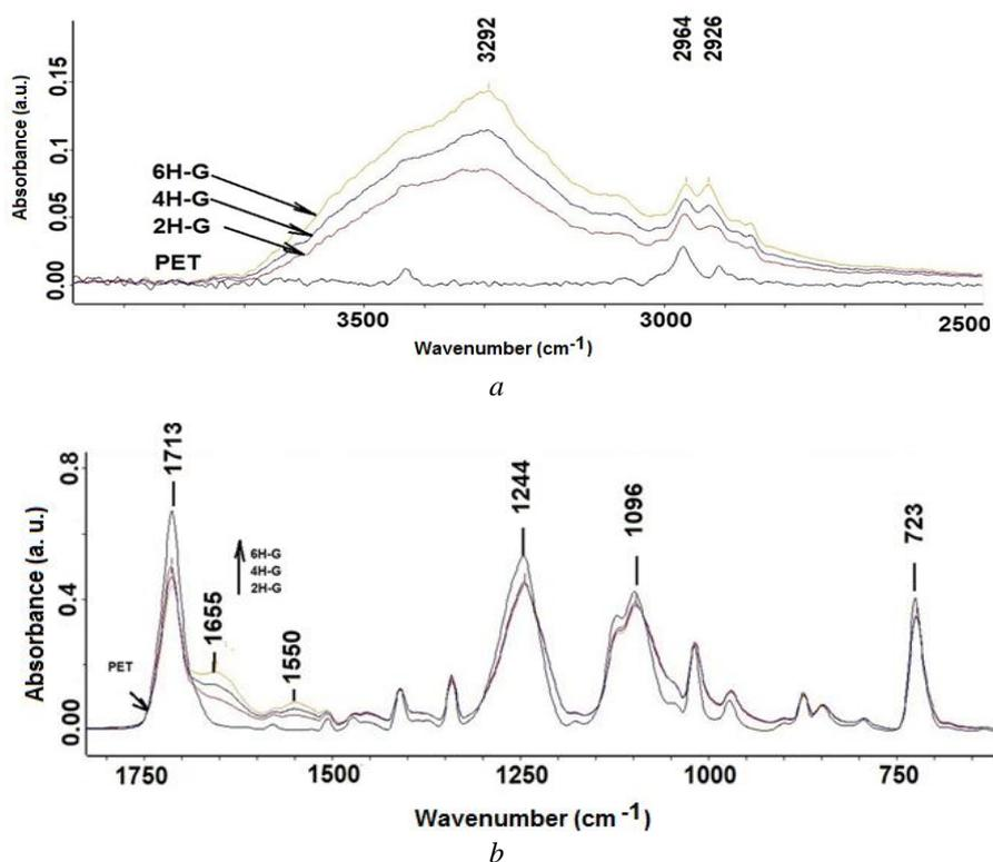
Fig. 4 – (a) and (b) are presented the FTIR-ATR spectra before and after immobilization with gelatine molecules.
