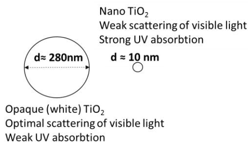
Fig. 5 – Optical properties of opaque and transparent nano-sized TiO 2 particles (Beetsma, 2017a).
