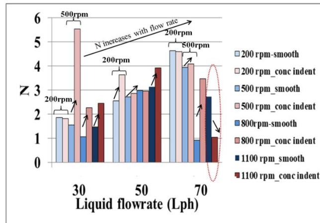
Fig. 5 – Comparison between smooth and concentric indented discs – N tanks-in-series model.
