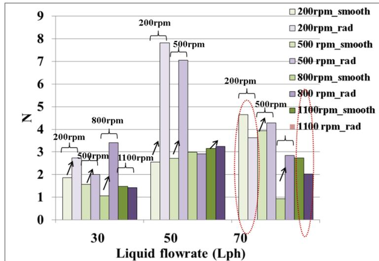
Fig. 6 – Comparison between smooth and radial indented discs, – N tanks-in-series model.
