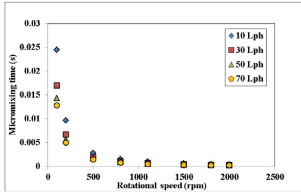
Fig. 4 – Micromixing time dependence on liquid flowrate and disc rotational speed.
