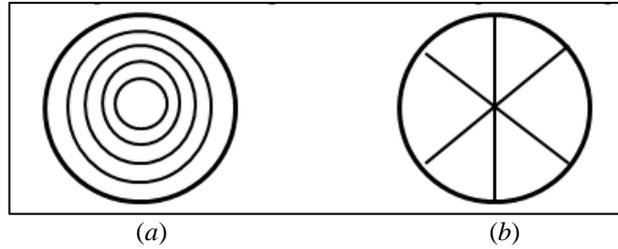
Fig. 1 – Sketch of the indented discs (a) concentric indentations; (b) radial indentations.
