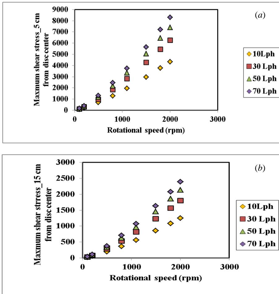
Fig. 2 – Dependence of maximum shear stress on liquid flowrate and rotational speed, at two different locations on the spinning disc (a) at 5 cm; (b) at 15 cm.
