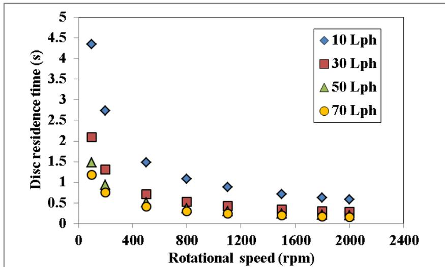
Fig. 3 – Residence time dependence on liquid flowrate and disc rotational speed.
