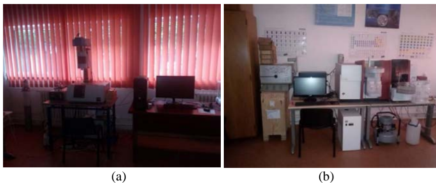
Fig. 1 – Netzsch Perseus STA 449 F3 gas chromatograph coupled gas chromatograph analyzer (a), Analytik Jena Zeenit 700 P atomic absorption spectrometer (b).
