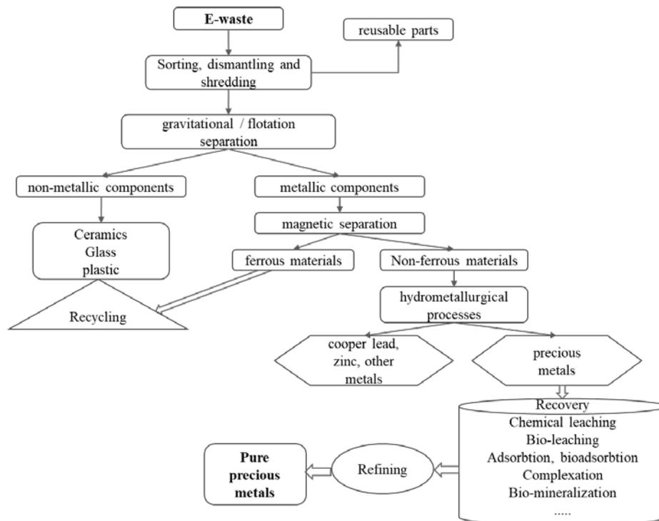
Fig. 2 – Block diagram for the recovery of precious metals from electronic waste.
