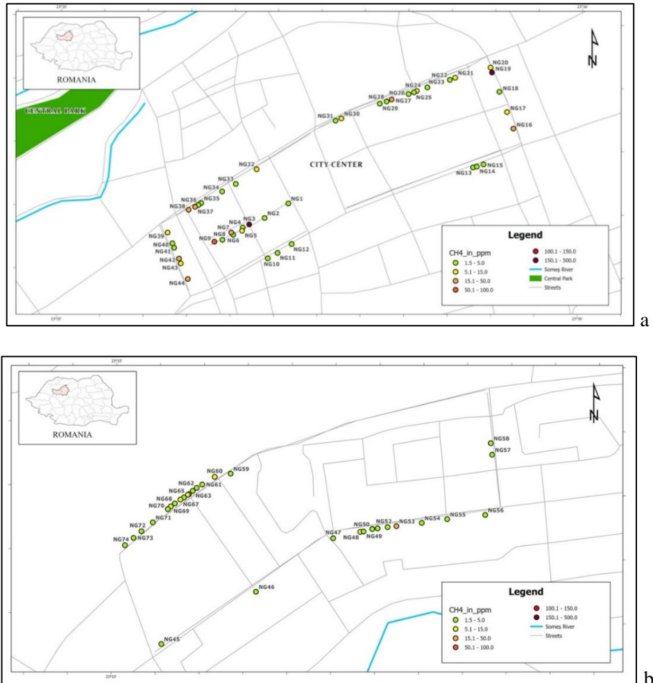
Fig. 3 – End-use points categorized according to the estimated value of CH 4 concentration (in ppmv). a) NG end-use points in the city center; b) NG end-use points in the residential neighbourhood.
