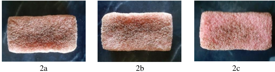
Fig. 1 – Appearance of self-compacting concrete specimens in the form of cubes and bars prepared for determining compression and flexural strengths 1a, 2a – version A; 1b, 2b – version B; 1c, 2c – version C.
