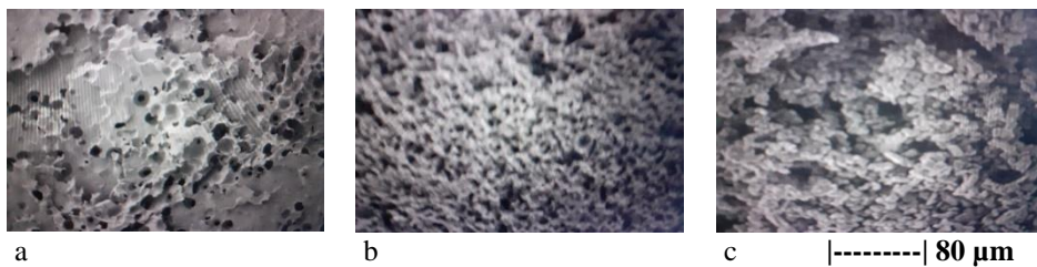
Fig. 2 – Microstructural images of self-compacting concrete specimens a – version A; b – version B; c – version C.
